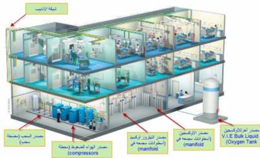
Figure 5-1 Medical gas Distribution in Hospital
