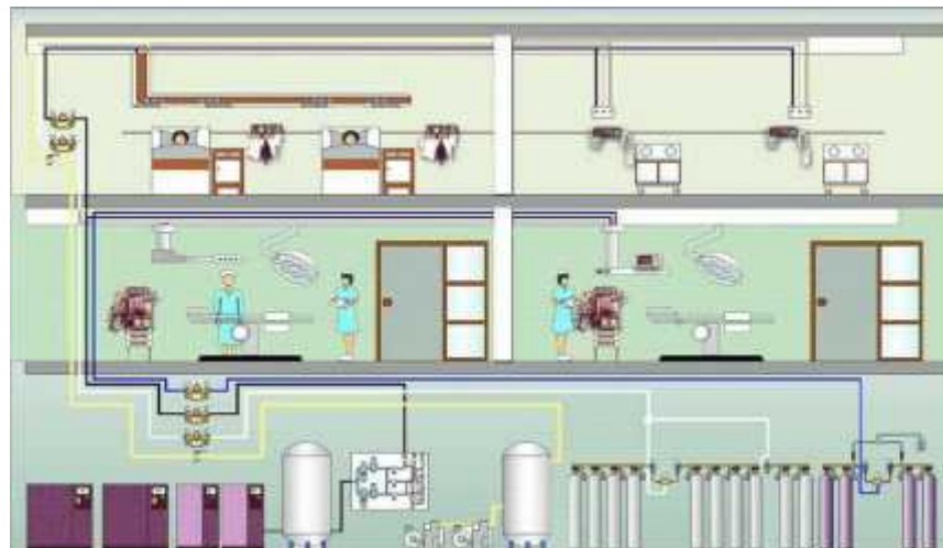
Figure 5-2 Medical gas Distribution in Hospital
