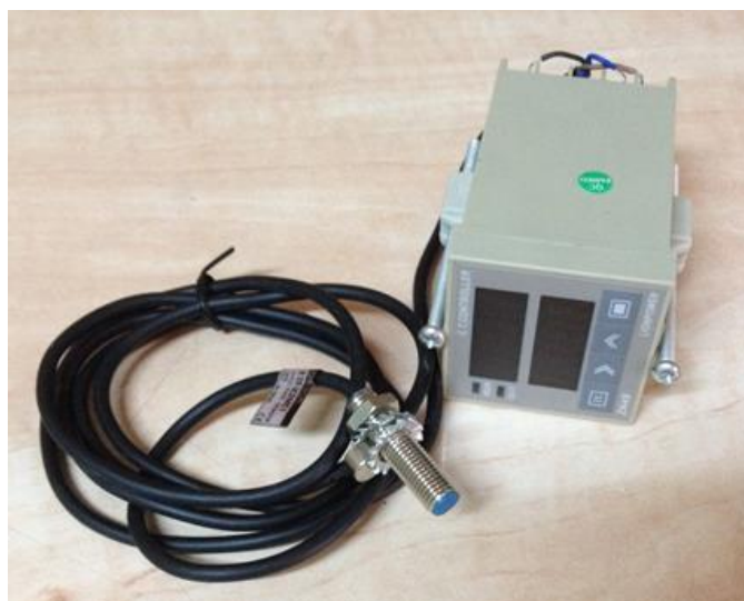
Fig.4.2: Rpm sensor with digital display screen
