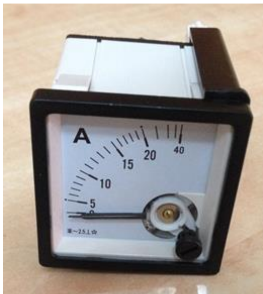
Fig.4.5: Mechanical ampere indicator
