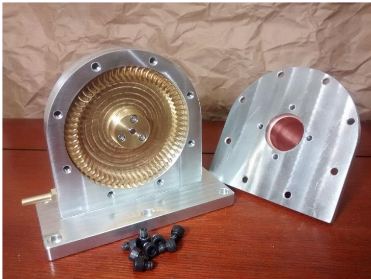
Fig.3.1.3: Simple impulse steam turbine
