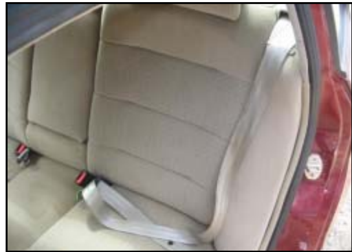
Figure 9. Rear left safety belt with fired pretensioner.
