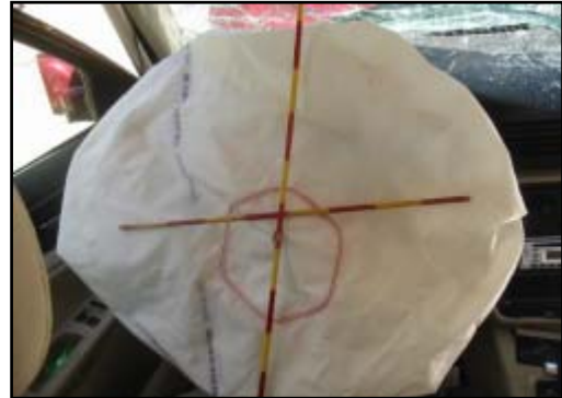
Figure 13. Deployed driver's frontal air bag.
