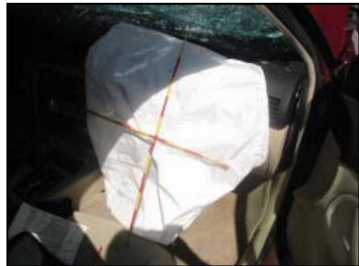
Figure 14. Deployed front right air bag.
