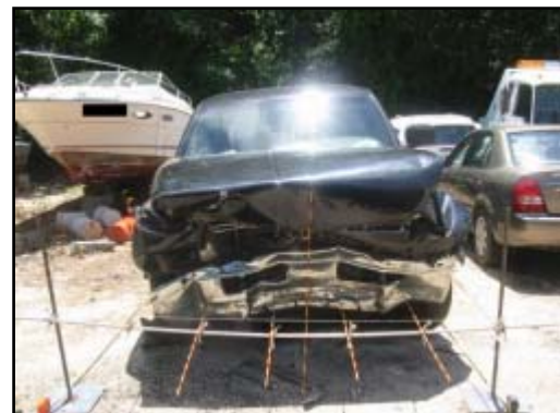
Figure 7. Crush profile for the 1999 Dodge Ram.
