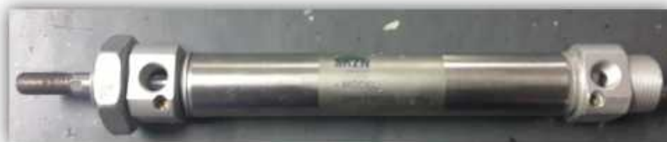
Figure 3.5 : The Double Acting Cylinder
