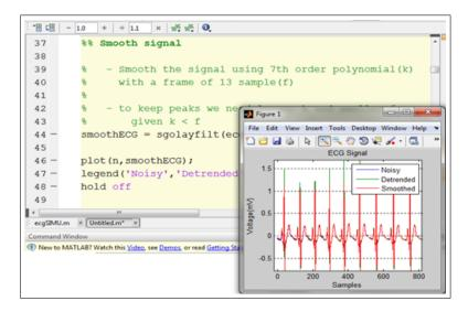
Figure 6.13: Smoothing ECG signal.
