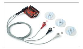
Figure 3.8: ECG electrodes with E-Health sheild.
