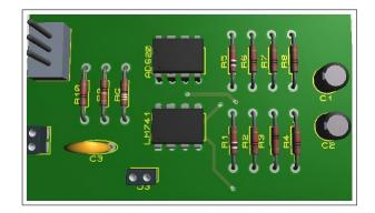
Figure 6.8: Complete ECG circuit.
