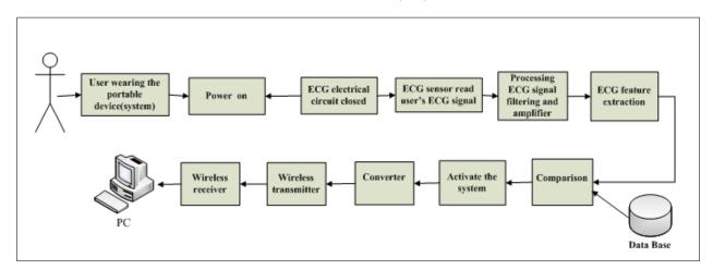
Figure 5.1: System block diagram.
