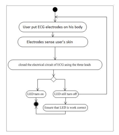
• figure(4.4) show activity diagram for closed ECG electrical circuit.
