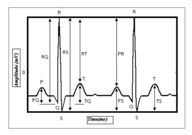
Figure 6.14: All amplitude features extraction.
