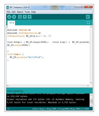
Figure 7.13: Bluetooth code test.
