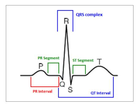
Figure 2.10: ECG segments and intervals[12].
