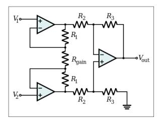
Figure 2.4: Typical instrumentation amplifier schematic.[11]
