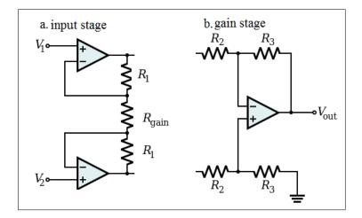
Figure 2.5: Input and gain stages of instrumentation amplifier.[11]
