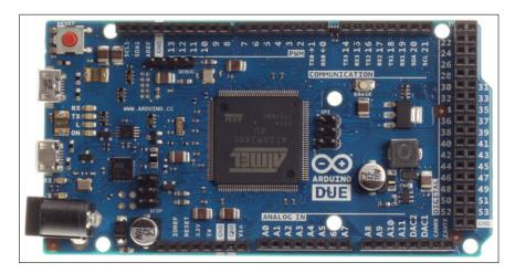
Figure 3.5: Arduino Due.
