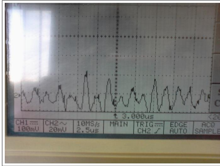
Figure 7.8: ECG circuit test.
