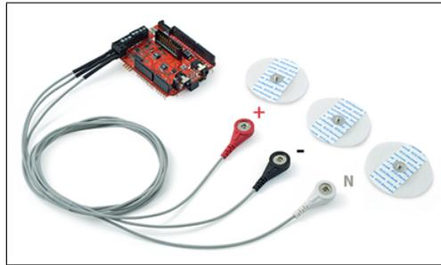
Figure 3.8: ECG electrodes with E-Health shield.
