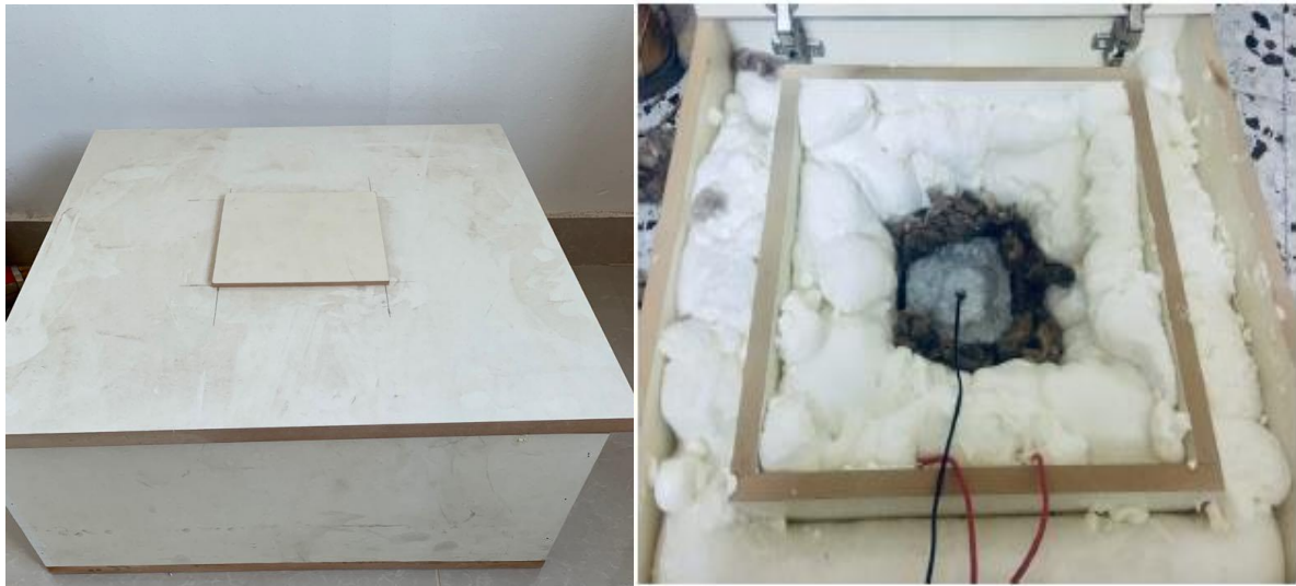
Figure 3.9: The hot plate thermal conductivity instrument [90].
