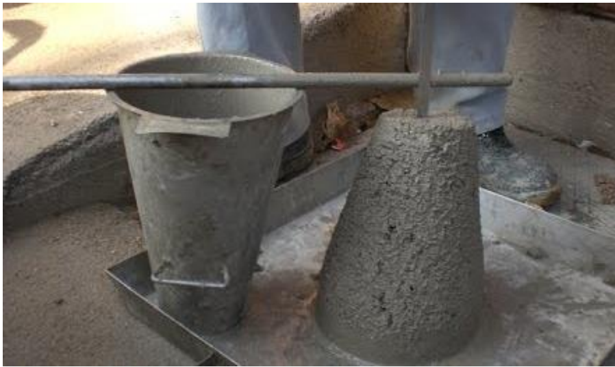
Figure 3.5: Slump test measurement.
