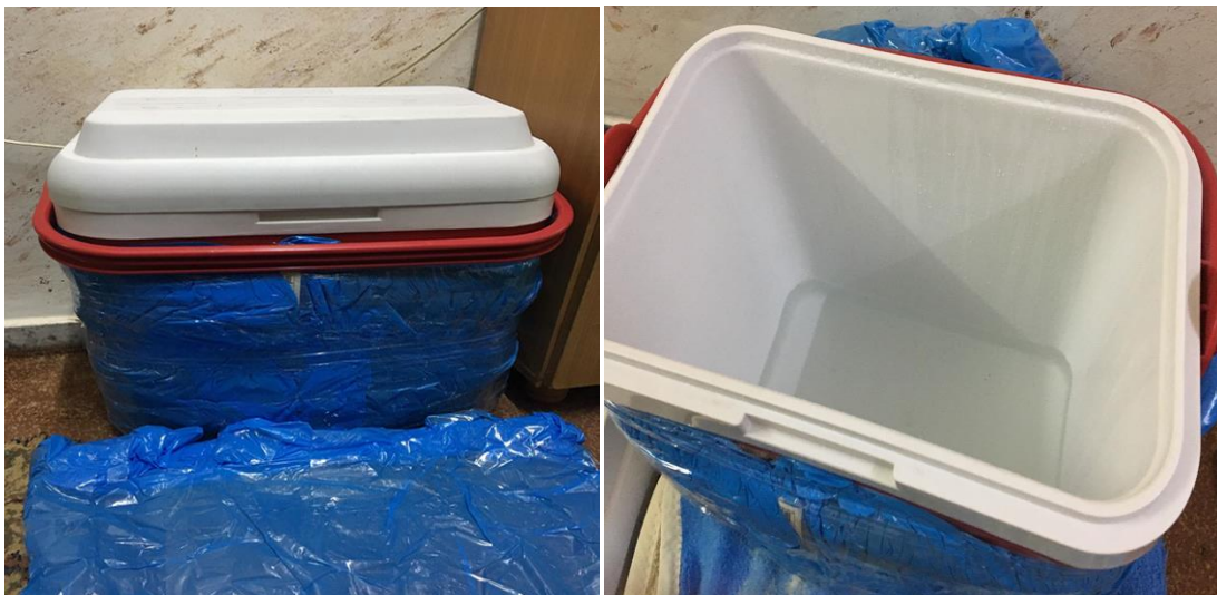
Figure 3.10: Foam box for measuring the specific heat capacity of concrete specimens [90].
