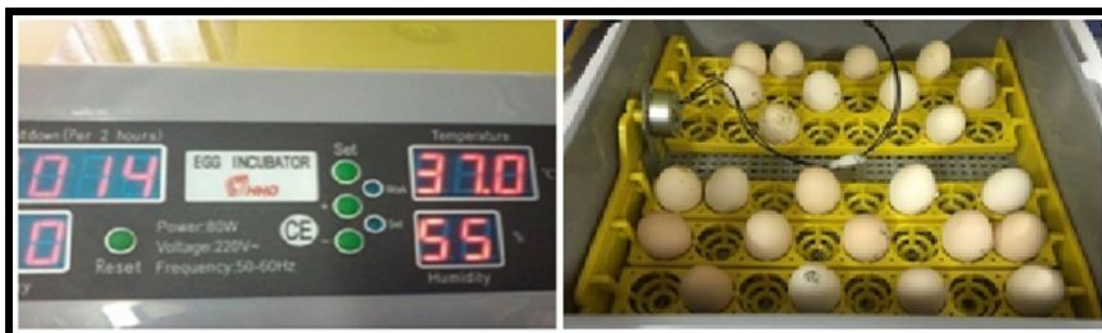
Figure 3.1: Egg incubator that moves the eggs by tilting automatically after the third day of incubation, with a temperature of 37^{\circ}\text{C} and humidity 55% - 60%.
