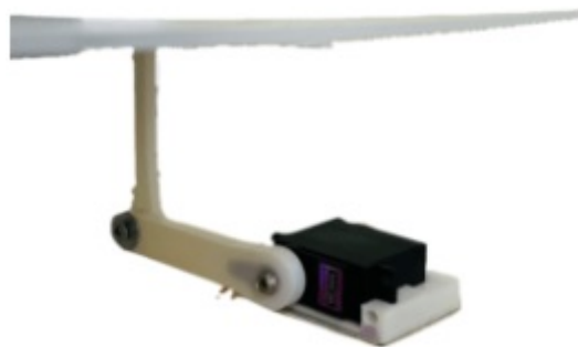
Figure 4.6: The link between the plate and the servo motor
