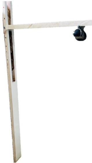
Figure 4.7: The logitech quickcam pro 9000 camera installed on the stand
