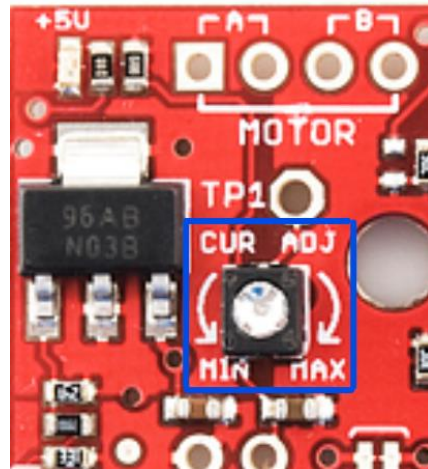
Figure 34: The potentiometer on EasyDriver chip
