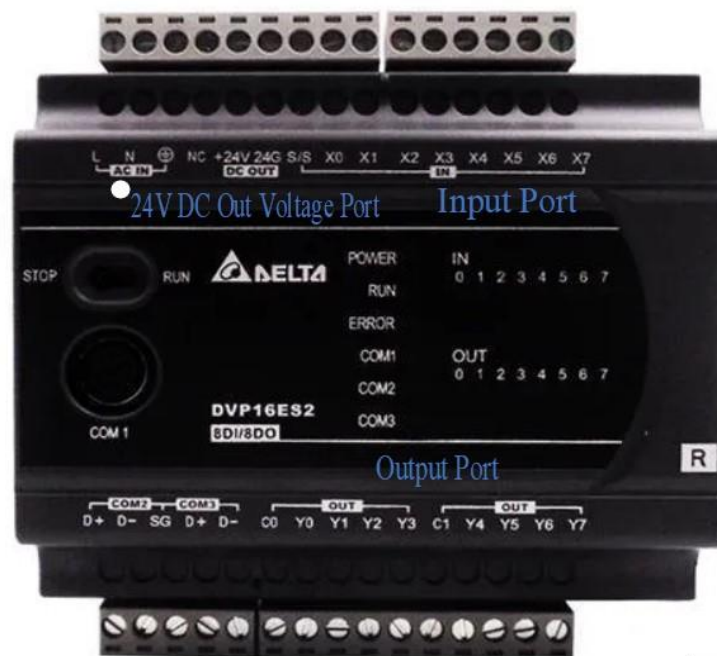
Figure (4.3): PLC Ports.
