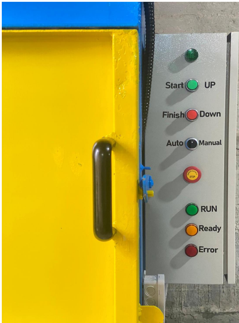
Figure (5.4): Machine Control Panel From Outside
