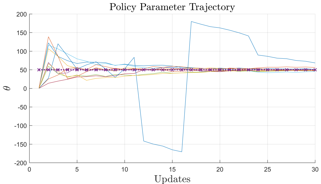
Figure 5.2: The trajectory of the parameter \theta through the co-adaptation process, where the \times -line represents the true twist value \beta_{twist} = 50
