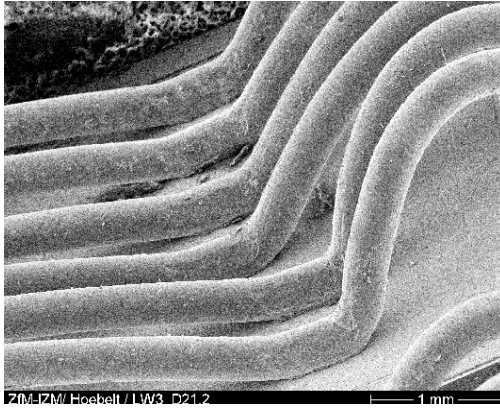
Fig.10: Bond wires of a diode power cycled at \Delta T_j=155K , no aging of bond wires is detectable
