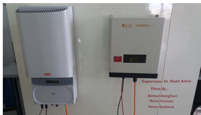
Fig.1: Inverters under Comparison (ABB left and OMNIA right) and Test Set-up
