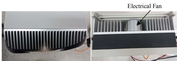
Fig.4: Cooling Systems of the ABB Inverter (left) and OMNIK Inverter (right)
