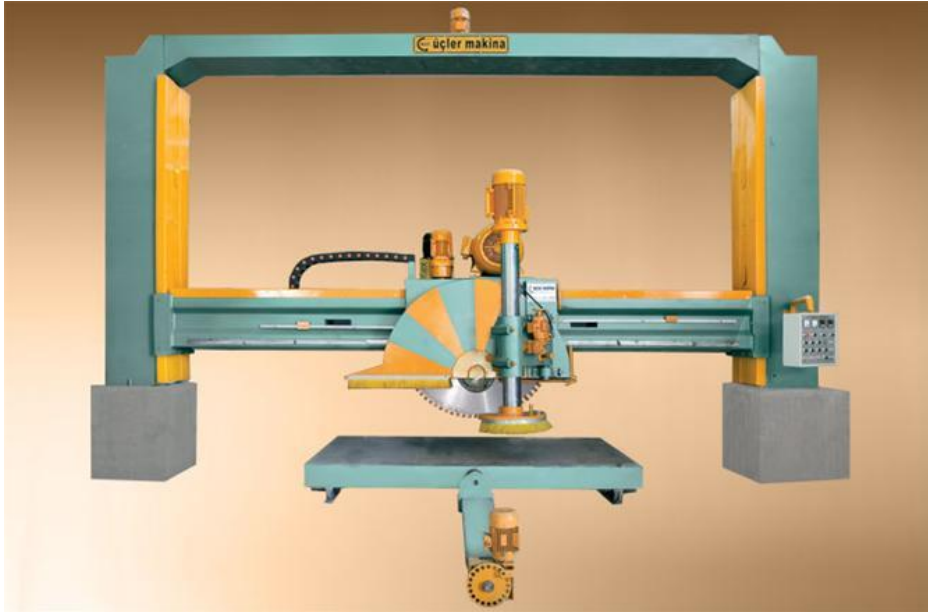
Figure (2.3): 2-D view of stone cutting machine
