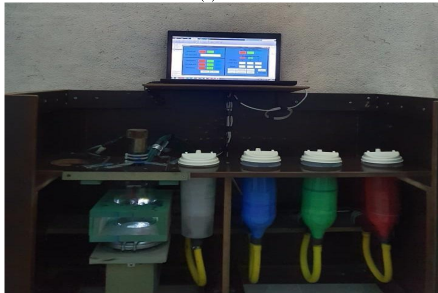
Fig. 3. Paints mixing equipment: (3a): Equipment setup, (3b): Lab-made equipment.
