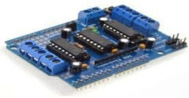
Figure 2.10 : L293D Motor Driver
