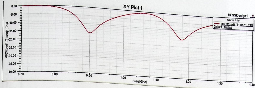
Fig 6.1: Return loss ( S_{11} - parameter in dB ) of the scaled dimensions for the E- shaped microstrip antenna with an air gap
