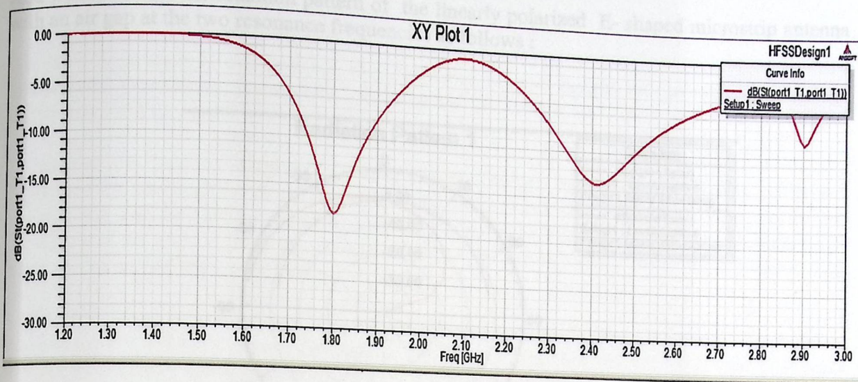
Fig 5.4 : Return loss ( S_{11} - parameter in dB) of the optimized dimensions for the E- shaped microstrip antenna with an air gap at ( 1800 & 2400 ) MHz .
