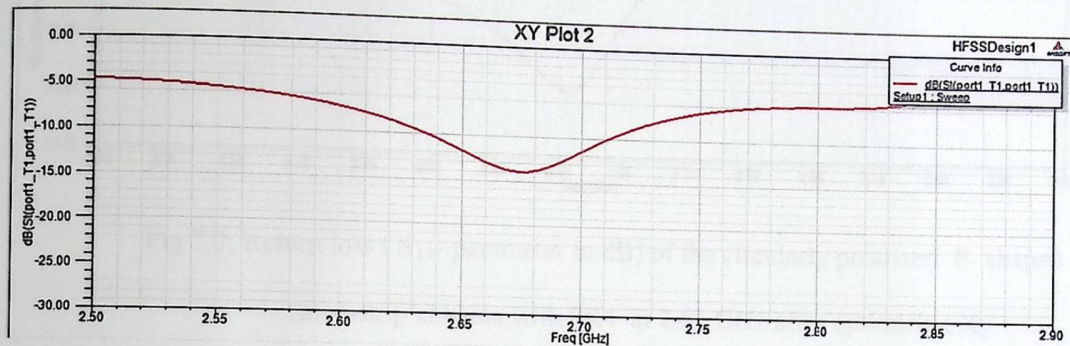
Fig 7.5: Return loss ( S_{11} - parameter in dB) of the circularly polarized E-shaped microstrip antenna with FR4 at 2.68 GHz
