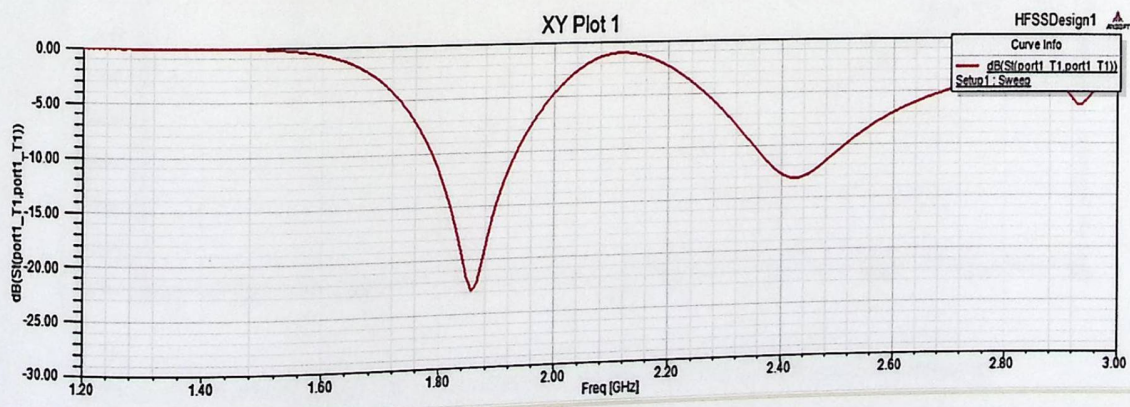
Fig 5.11: Return loss ( S_{11} - parameter in dB) of the E- shaped microstrip after decreasing W_s
