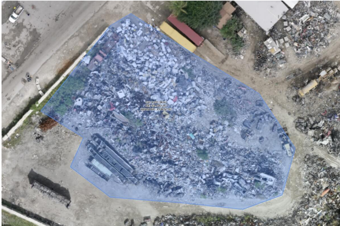
Figure (2-8) : volume measurement of a landfill in the Bahamas
