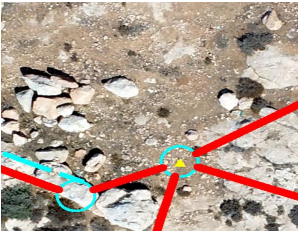
Figure (5-3) : Check points and their locations on the ortho photo
