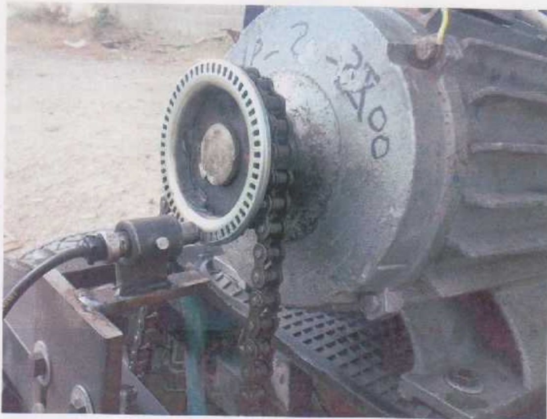
Figure 7.26: Inductive speed sensor and teeth connected with gear in electric motor
