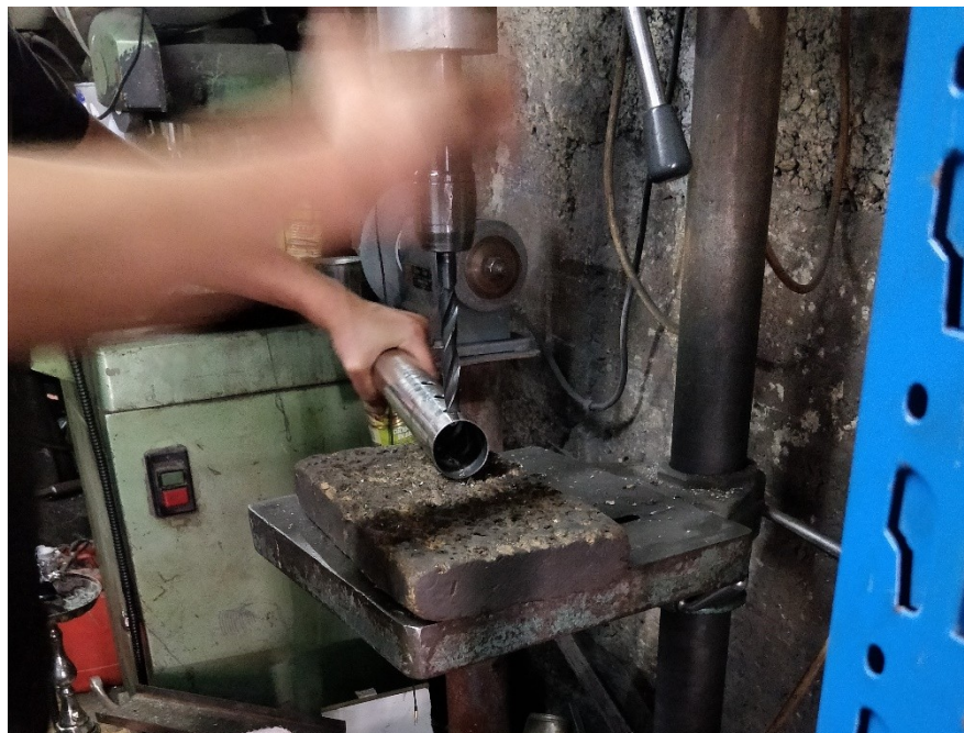
Figure 3.24: Holes Drilling Through the Pipe
