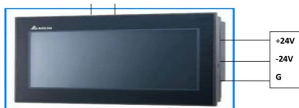
Figure 17 Touch screen (HMI)
