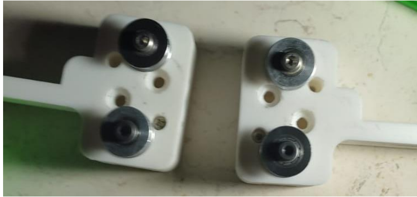
Figure 5-26: Smooth pulleys installed on the brackets
