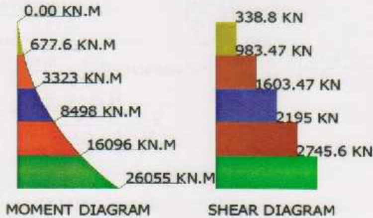
Fig.(4.0) Shear and Moment Diagrams
