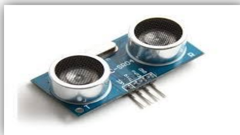
Figure 7: Ultrasonic Distance Sensor. Source [17].
