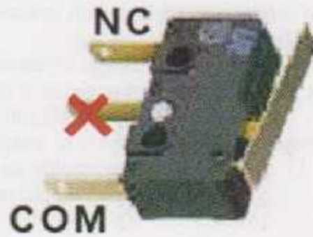
Figure (4.31): Limit switch terminals are used and not used.
