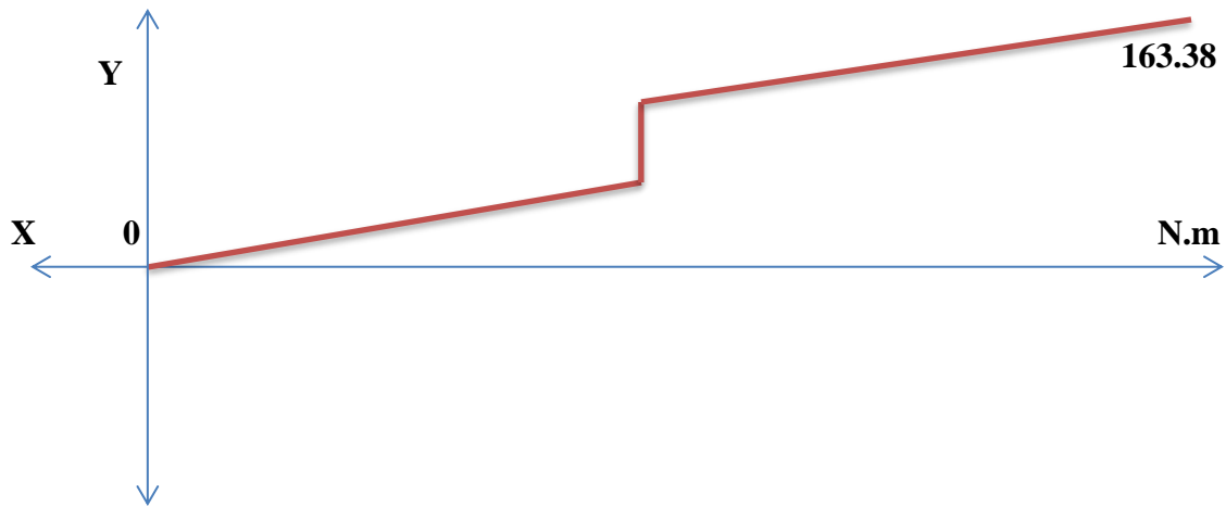
Figure 6-9 : Bending moment diagram ( M )
