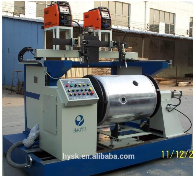
Figure 3-4 : Automatic arc welding machine[8]
