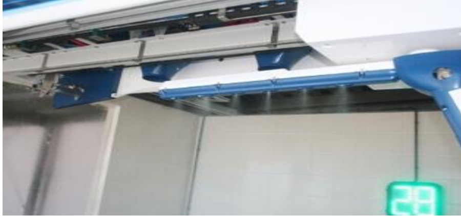
Figure 2-3 Sprayed water by smart 360° rotate arm[10]
