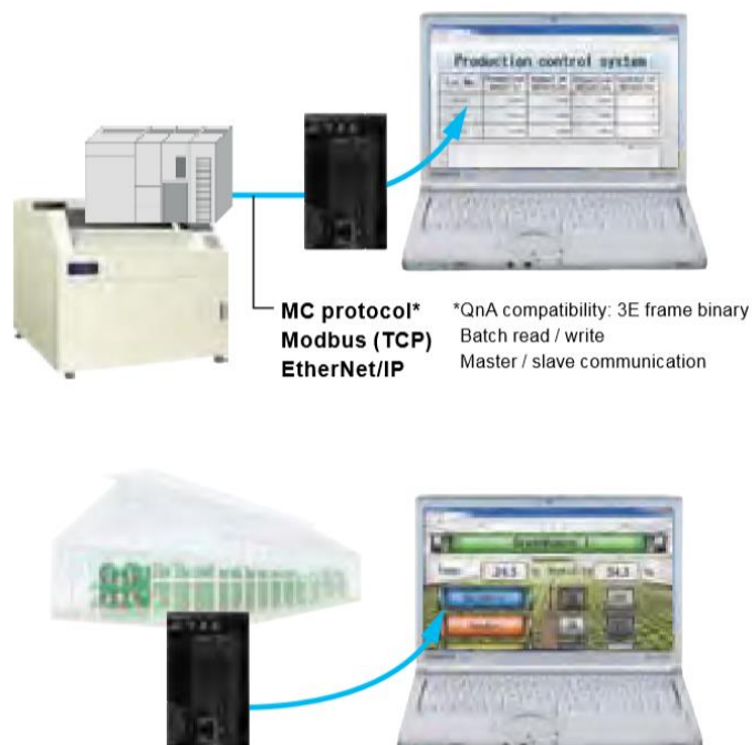
Figure 0.10 Local & remote connectivity [25]
