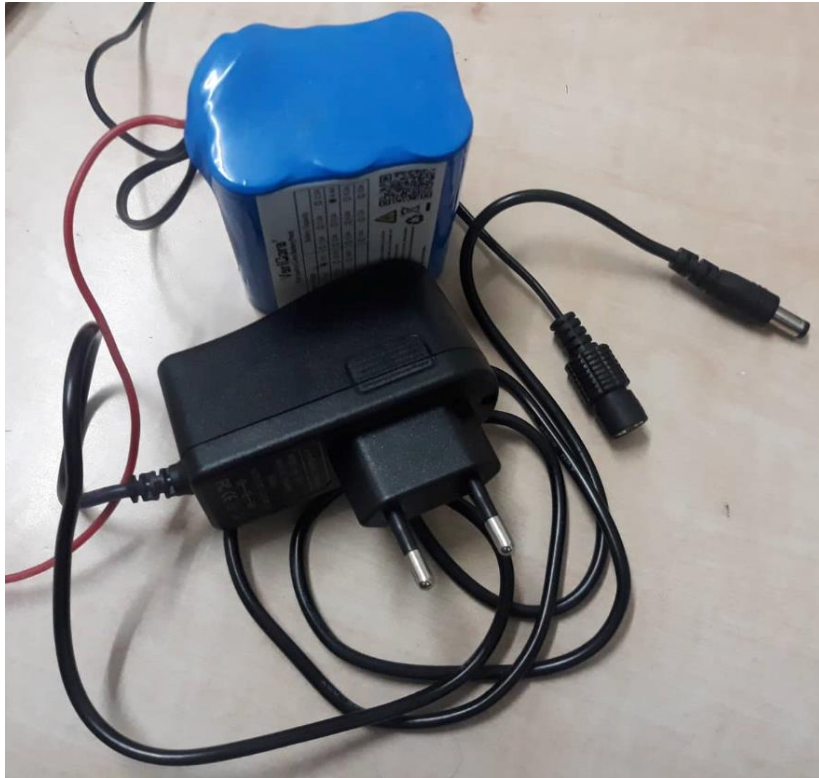
Figure 5.18 Charger of the 12V battery
