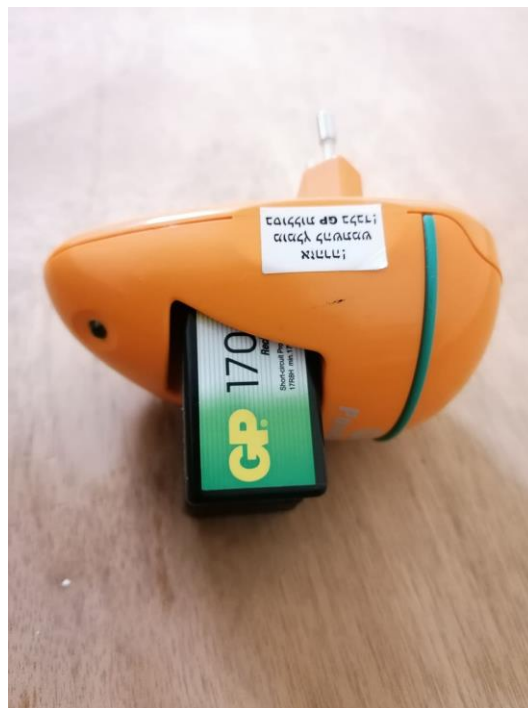
Figure 5.19 Charger of the 9V battery
