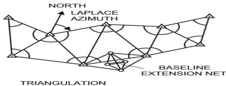
Figure (2.2): Triangulation with baseline extension net and Laplace azimuth (principle). [5]
