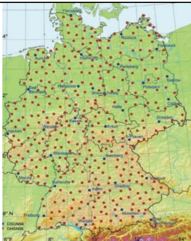
Figure (2.19): Primary gravity net (red circles) of Germany. [3]
