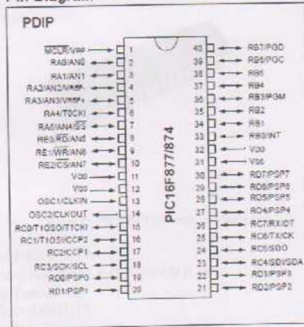
Fig4.2: PIC16F877 microcontroller Pins
