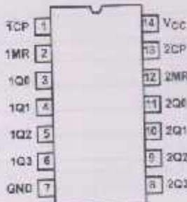
CD74HC393, CD74HCT393 (PDIP, SOIC) TOP VIEW
