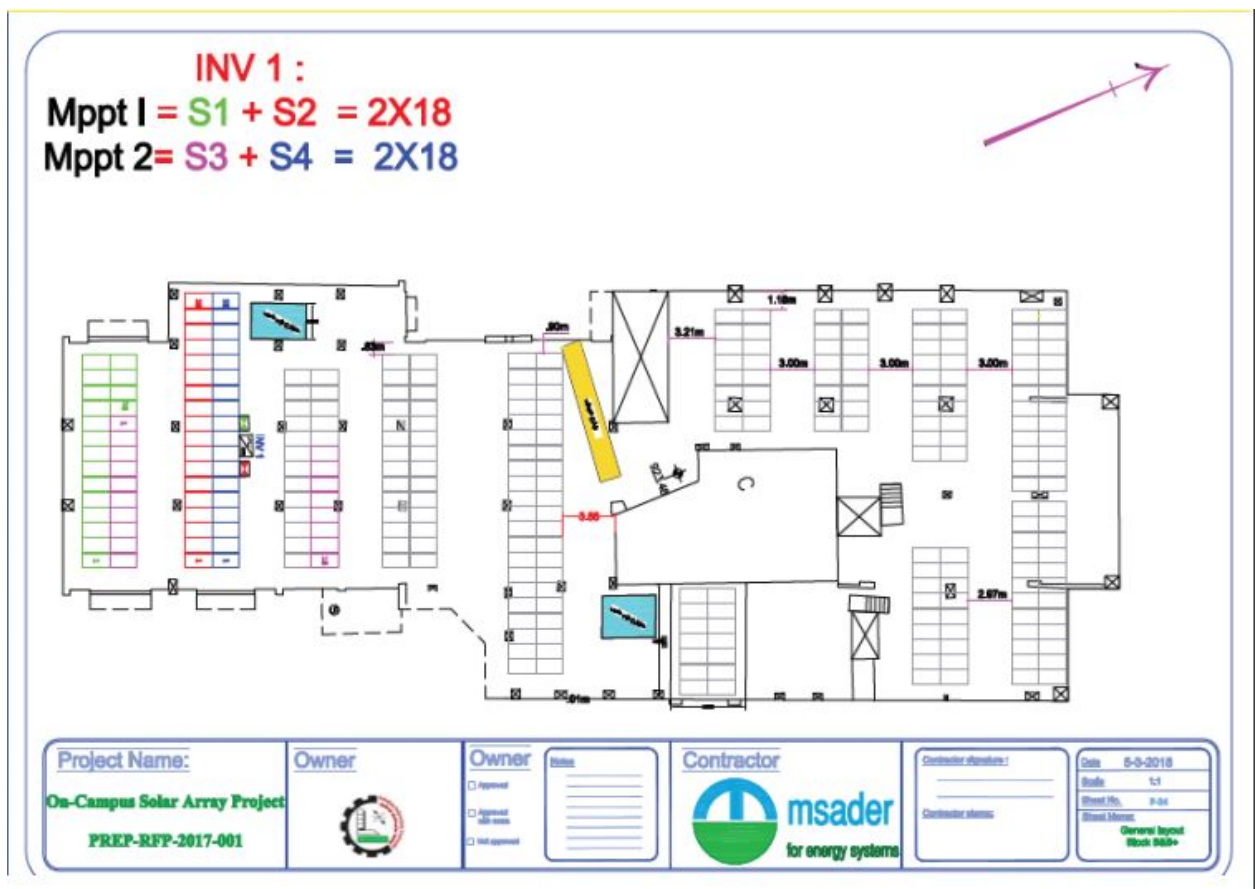
Figure A.6: Distribution of photovoltaic cells on the Inverters for a building B&B+
