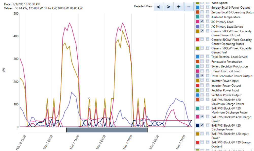
Figure 5.11: Output of PV-Wind Turbine-Diesel Generator and Battery bank
