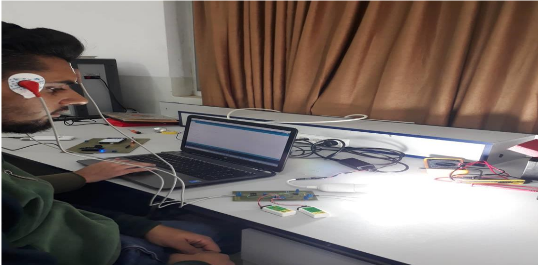
Figure 5 5: EOG circuit with light.
