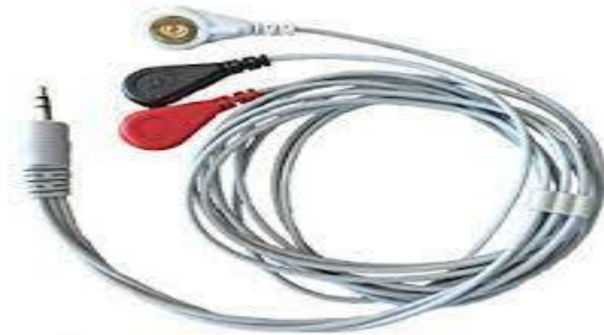
Figure 3. 4: Ag/Ag cl electrode
