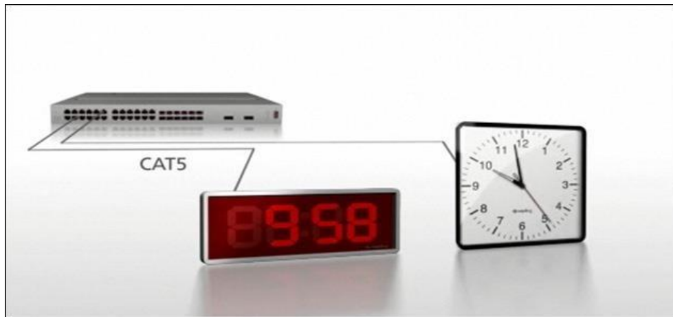
Figure 6.5 IP Master Clock System
