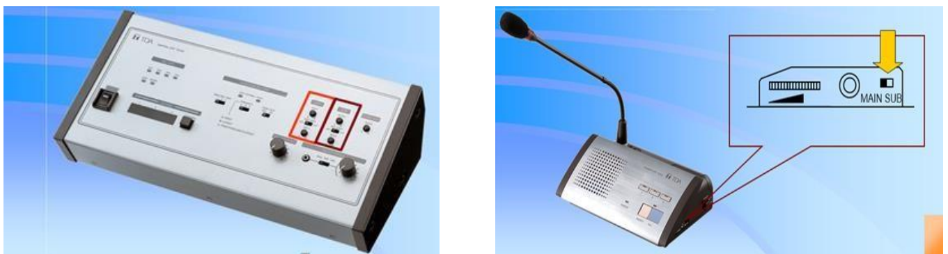
Figure 2.24 Main & Sub Channel
