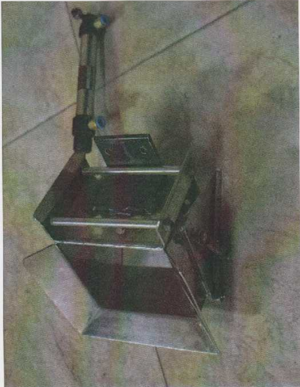
Figure (5.5): The Feed Hopper
