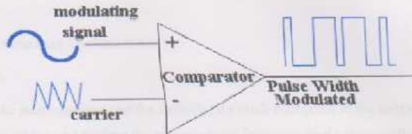
Figure 3.7 Generation of PWM sinusoidal using comparator
