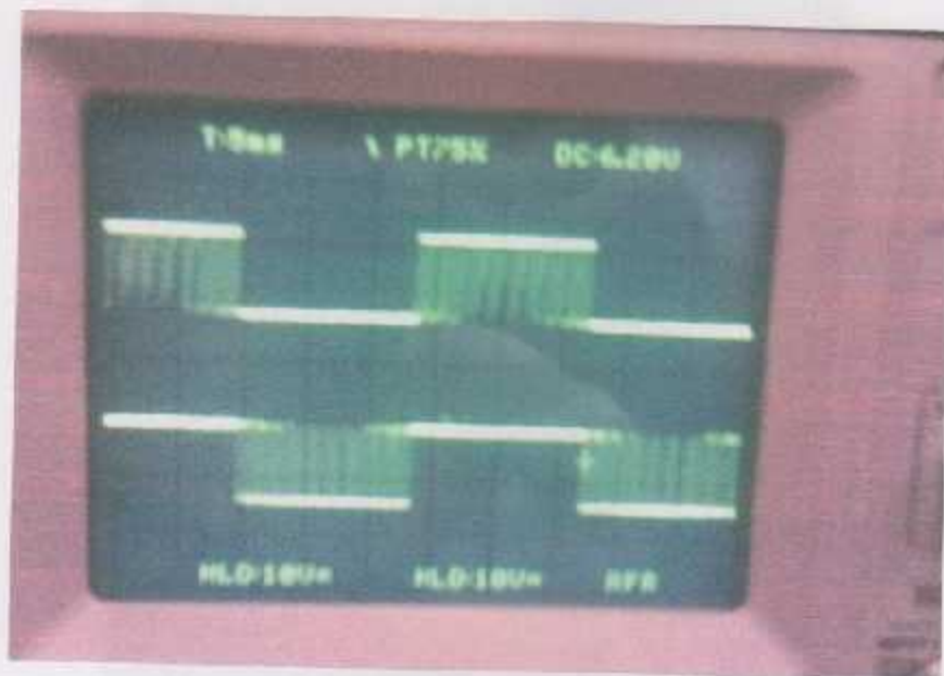
Figure 5.13 : PWM Signals (Gates Signals)
