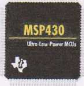
Figure(4.16): MCU with 14 bit ADC
