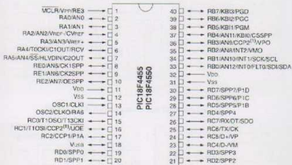
Fig.(4.18): PIC 18F4550 pin out
