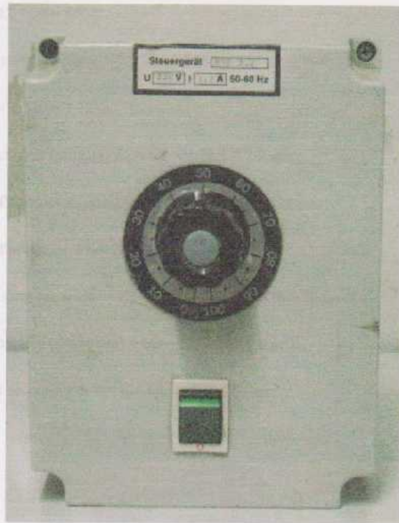
Figure 4.8: Outside control platform of a Variac transformer.
