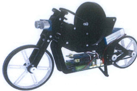
Figure 1.2: A self-balancing motorcycle[2]
