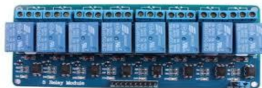
Figure (3.5) Relays PCB
