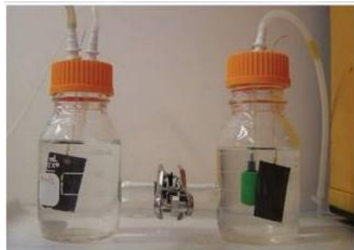
Figure 3.18: The conventional H-design MFC [41].
