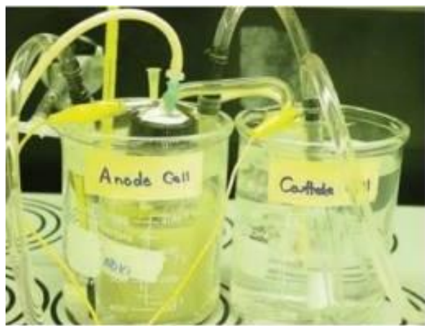
Figure 3.21: A salt bridge MFC [41].
