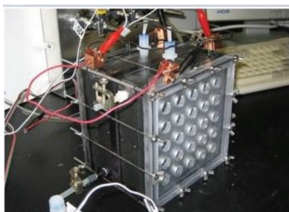
Figure 3.22: MFC with cells joined in series [41].
