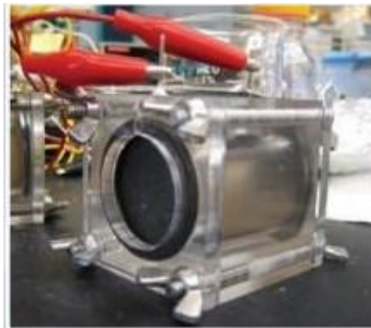
Figure 3.20: A single chamber air cathode system [41].
