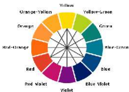
Figure (4.5): Complementary colour: If the solution has one of the colours it will absorb the obverse colour.
