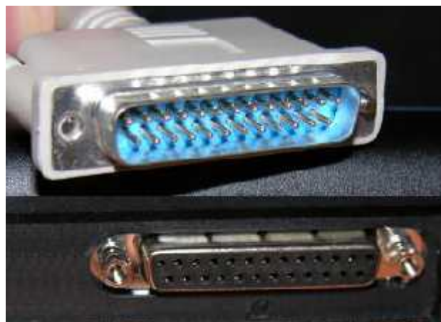
Figure (5.18): Data cable.
