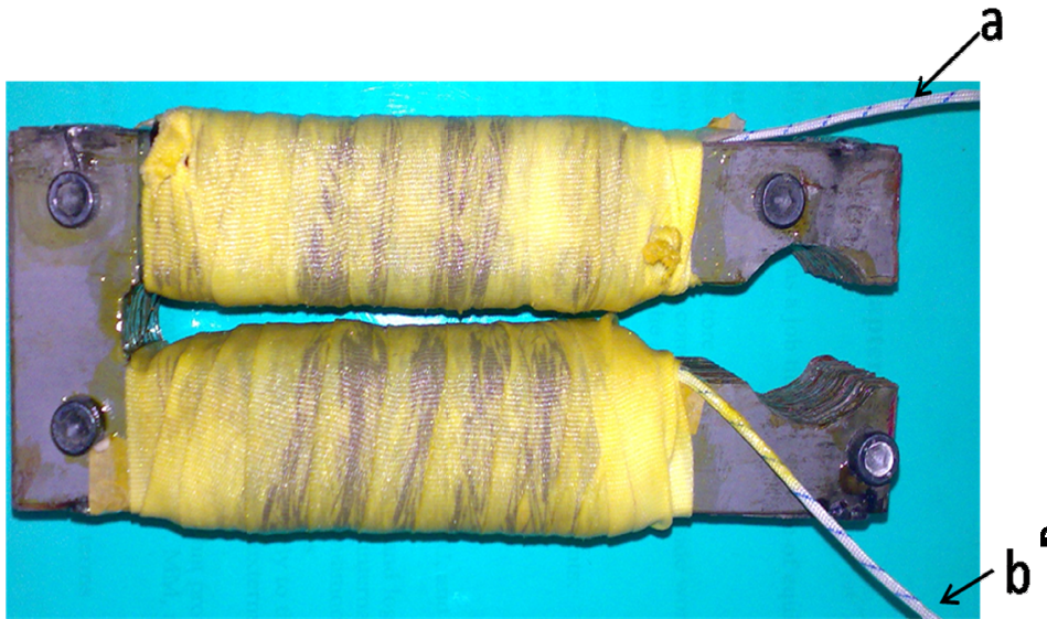
Fig 4.7: (a) starting point of windings (b) ending point of windings (practical)
