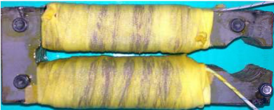
Fig 4.4: Stator windings (practical)
