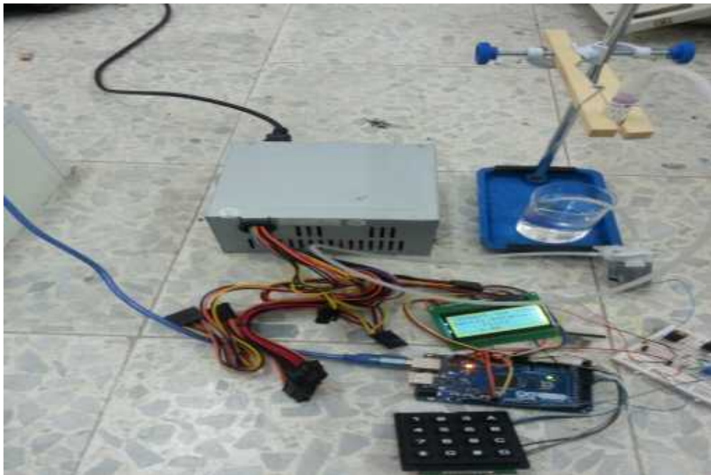
Figure (5.1): testing of first part of project(pump,Arduino,keypad,LCD)
