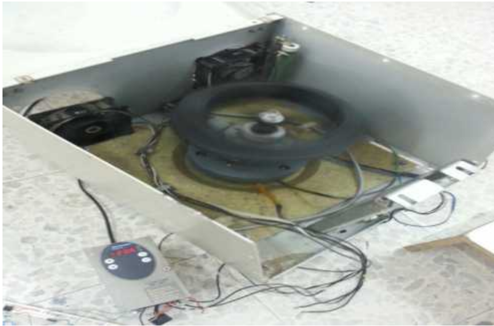
Figure (5.6): Centrifuge system motor
