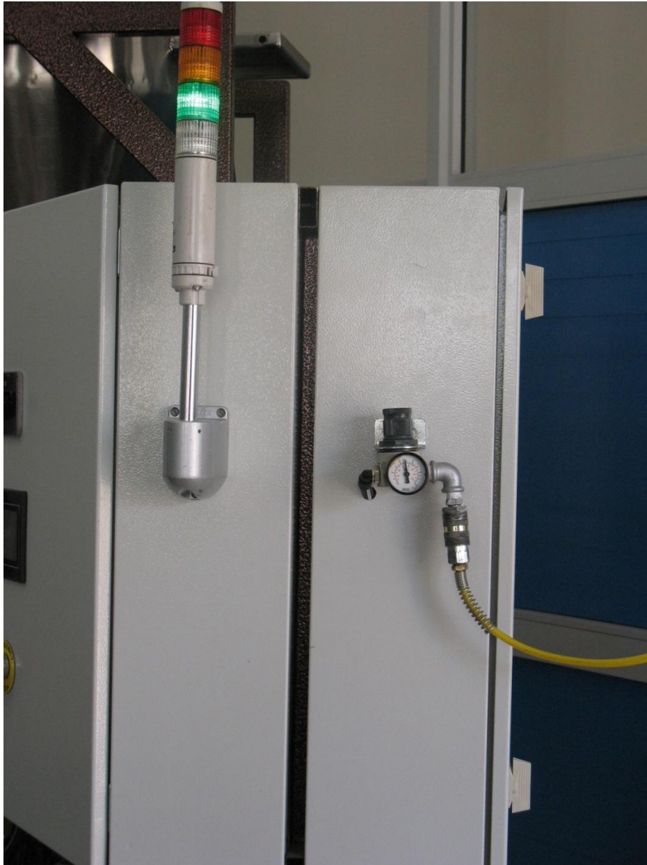
Figure (4.22): Indicator Lamp and Pressure Regulator of the Machine
