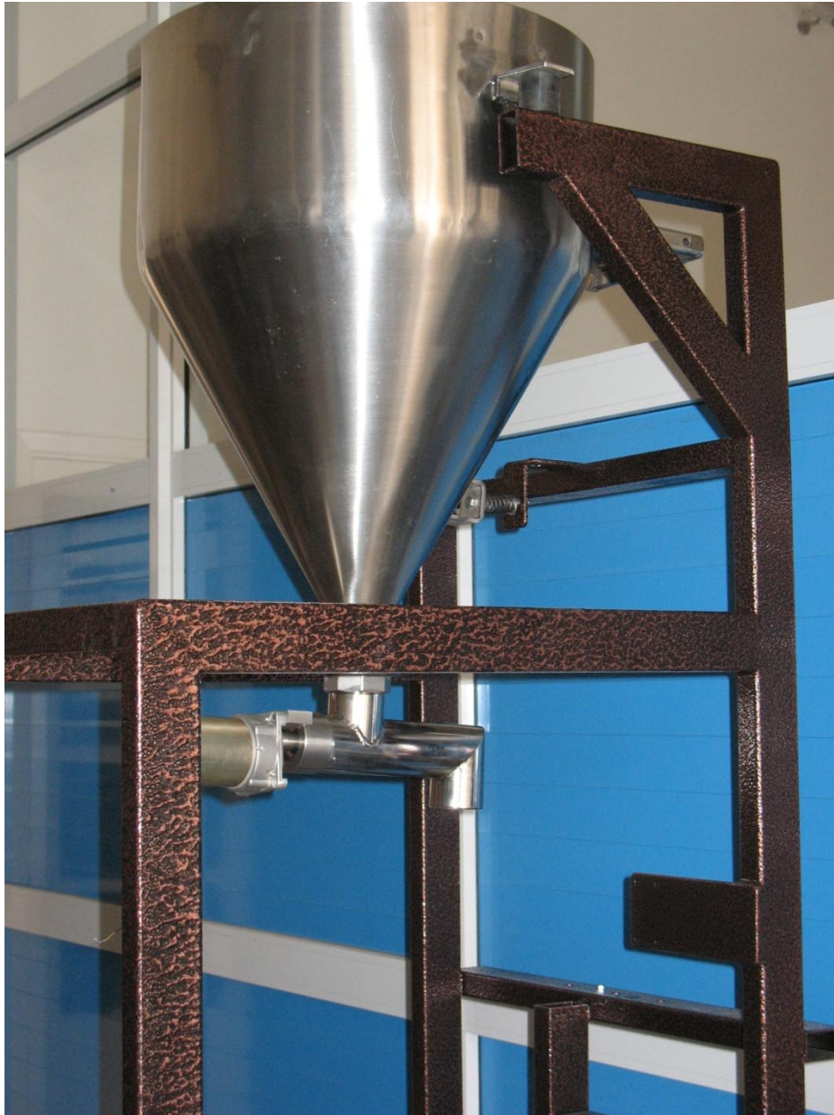
Figure (4.6): Screw Connection with The Hopper
