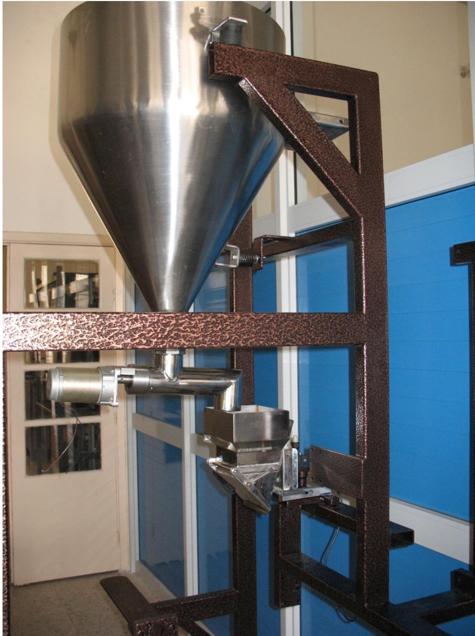
Figure (4.9): Weight Scale Connection with the Body of the Machine
