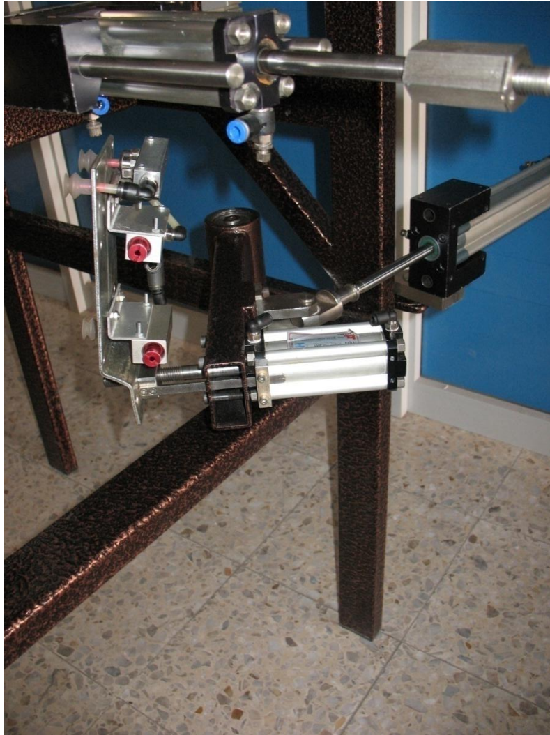
Figure (4.13): Vacuum Unit Device Connection with the Body of the Machine (From the Right-Hand Side)
