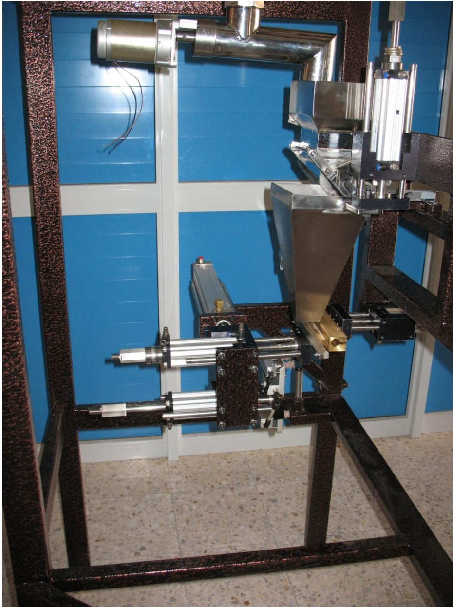
Figure (4.16): Vacuum Unit Device Connection with the Body of the Machine
