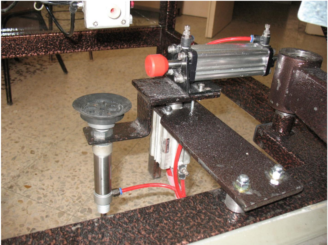
Figure (4.19): Drum Cylinder Connection with the Body of the Machine
