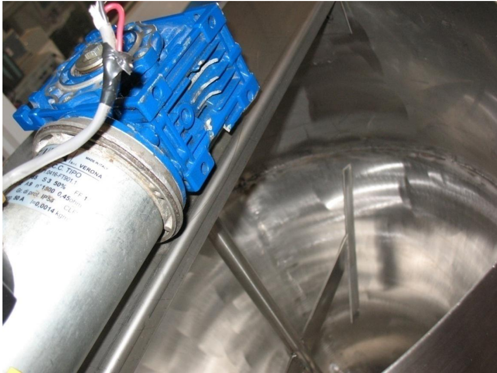
Figure (4.4): Mixer Blades inside the Hopper
