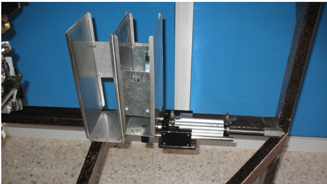
Figure (4.18): Bag Container Connection with the Body of the Machine
