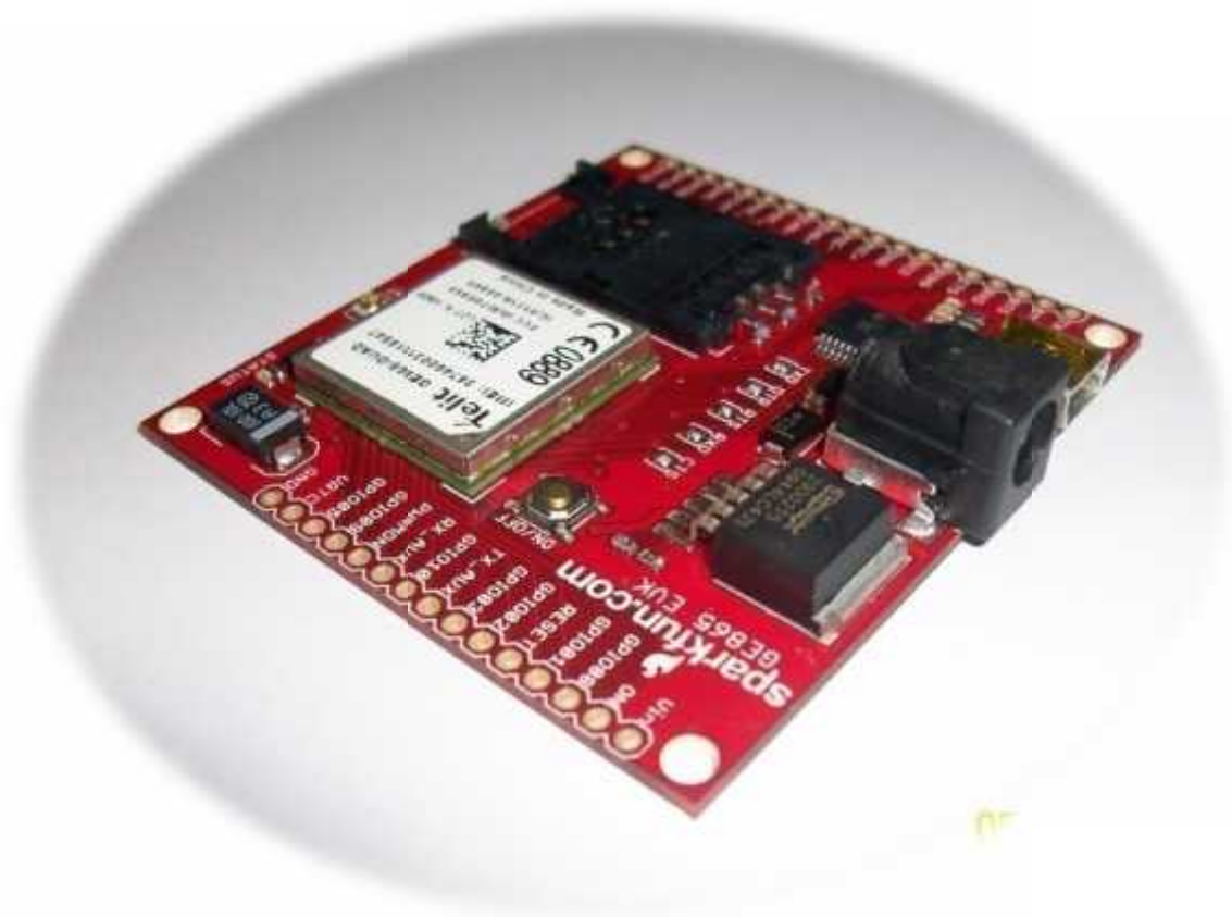
Figure 4.5: overview of GE-865 EVKGSM Modem
