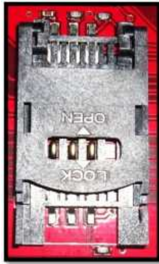
Figure 4.10: SIM Card holder
