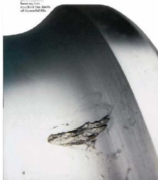
Figure7: Bearing failure because normal fatigue failure
