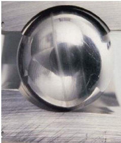
Figure8: Bearing failure because reverse loading
