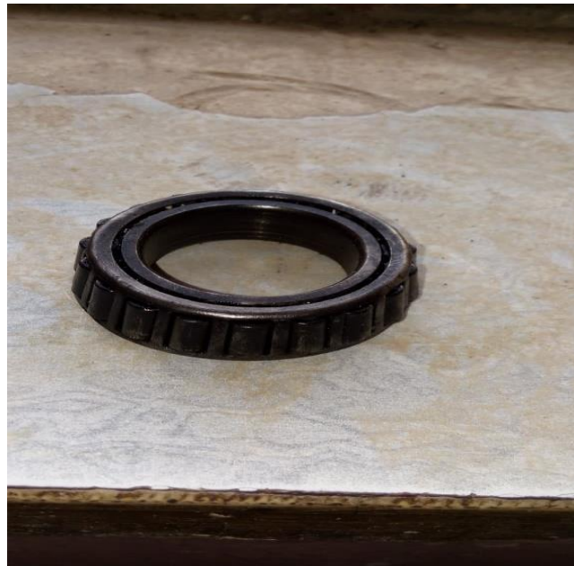
Figure 31: Bearing with dirt lubrication
