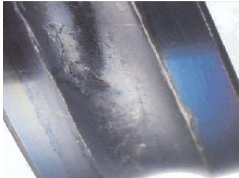
Figure10: Bearing failure because lubricant failure
