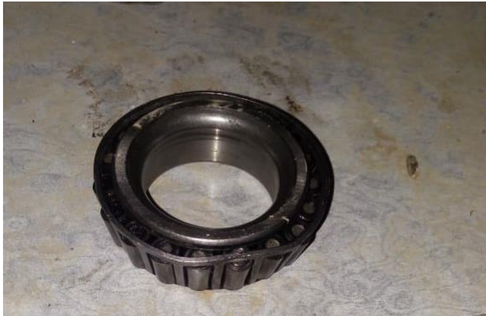
Figure 35: Bearing inner race failure
