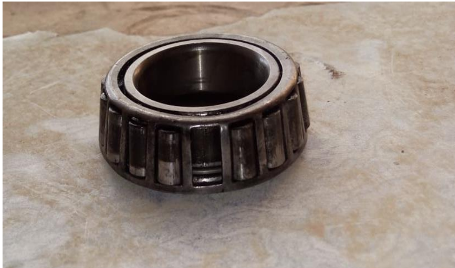
Figure 33: Bearing without one roller
