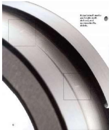
Figure5: Bearing failure because false brinell
