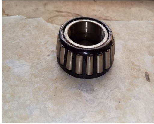
Figure 27: Healthy bearing with lubrication
