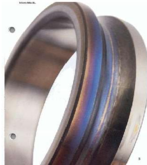
Figure4 Bearing failure because overheating
