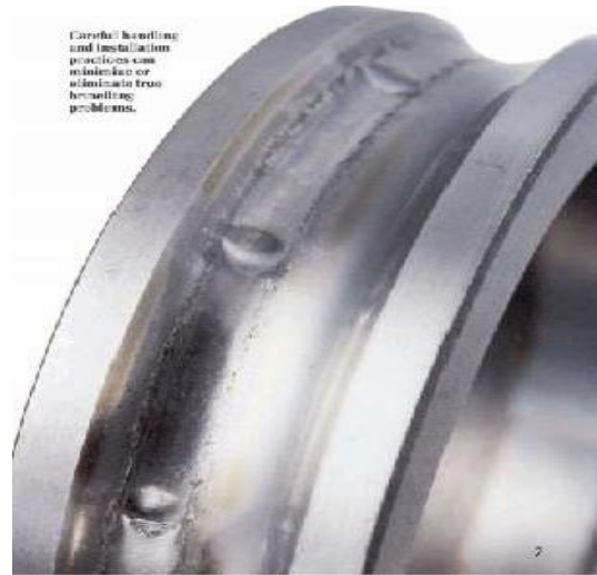
Figure6: Bearing failure because true brinelling .
