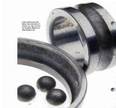
Figure 11: Bearing failure because corrosion
