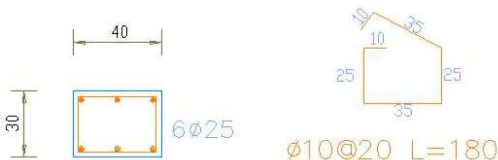
Fig.(4.10): Detail Of Column.
